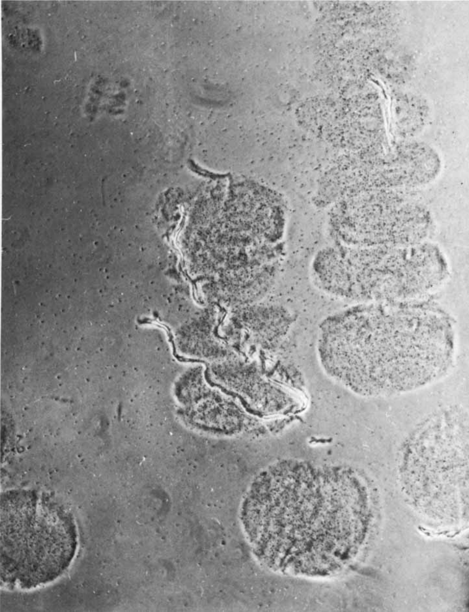
Fig. 2. Photomicrograph ( \times 120 ) of polyester yarn heated to 200^{\circ}\text{C} in a texturing machine (no false twist) and swollen in 83% (v/v) dichloroacetic acid/water solution.
